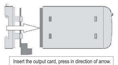
6) After inserting the output card insert the Interface card PCB and back cover.
