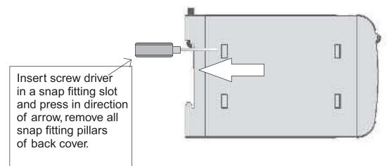
3) Remove the back cover and take the Output card out.
